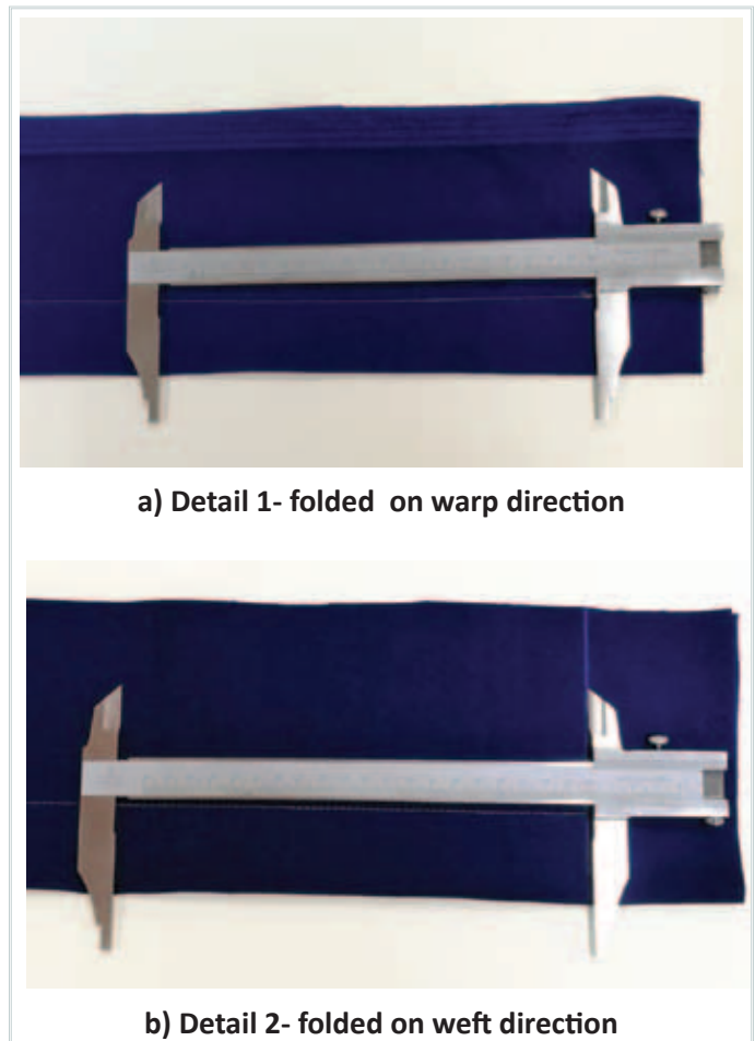
Fig. 1. Stitch length 3 stitches/cm
