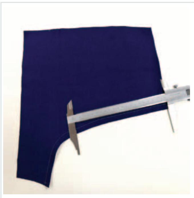
Fig. 3. Assembled details 5 and 6 , stitch length 4 stitches/cm
