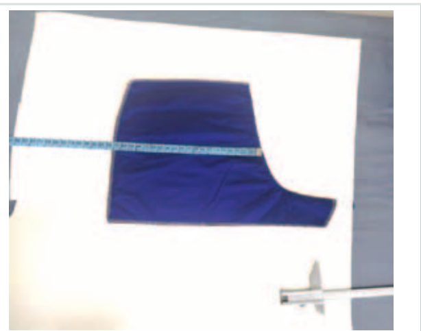
Fig. 6. Deformation of the assembled details 5 and 6 after treatment
