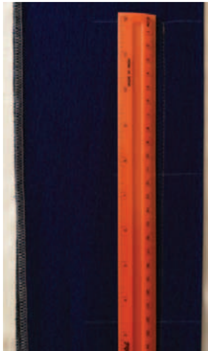
b) Detail 4 before and after treatment - tensile Fig. 8. Deformation of assembled details- elongation 10%
